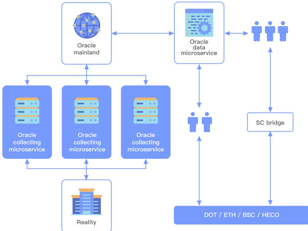
The LON system adopts a layered modular micro-service architecture, which divides the predictive machine network into three modules:
